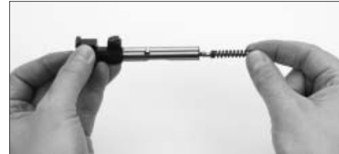
illu. 50) Install firing pin Correct location of retention stud notch
