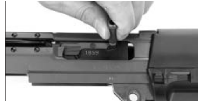
illu. 42) Use cocking handle to slide bolt to rear
