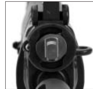
illu. 31) Gas valve in position I
