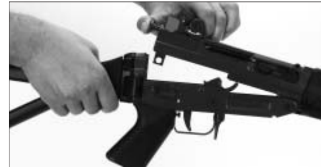
illu. 40) Remove trigger housing
