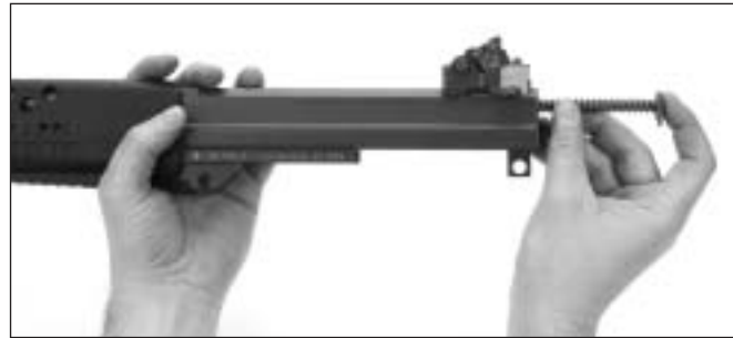
illu. 53) Inserting recoil spring and guide
