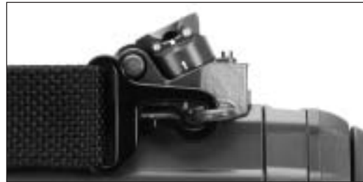
illu. 38) Sling attachment to the butt stock
