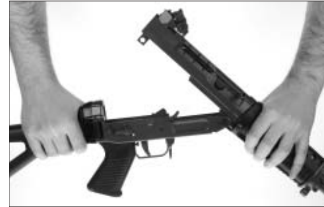
illu. 54) Installing trigger housing
