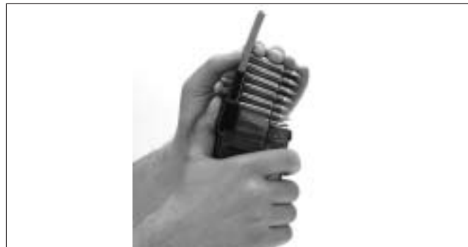
illu. 22) Loading the cartridges into the magazine by means of the loading tool
