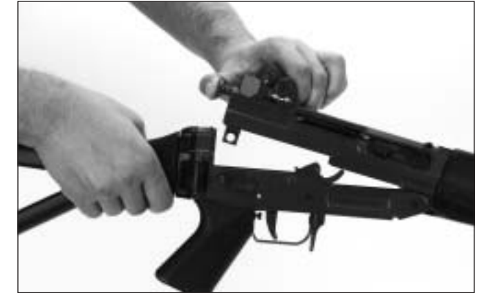
illu. 55) Installing recoil spring
