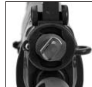
illu. 32) Gas valve in position II
